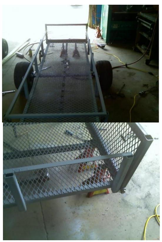
I reused old axle of the old trailers we have around . Found out that the club car wheels fit on them . So about 200 \$ + 40\$ paint and welding rods .the mesh metal was only 90\$ for a 4 x 8 ' sheet .
